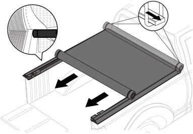
• Snap the tail lock into the lock groove of the side rails as shown
