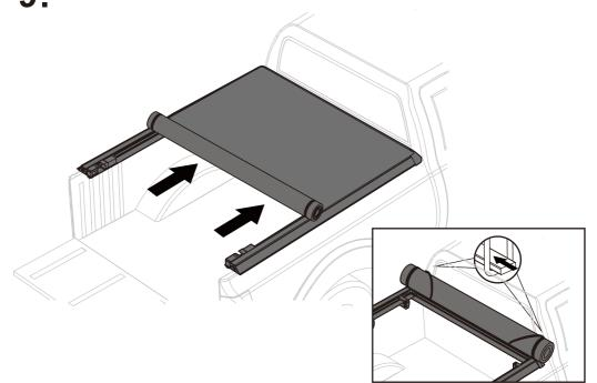
• There is a scale label on the tail of the side rail. If you find that the bed cover tarp is loose, you can move the tail lock backwards according to the situation. Will make the tarp tighter.
