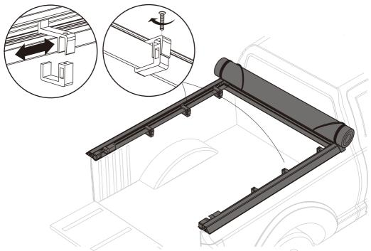
• Untie the spring cords on both sides of the bed cover and unfold the bed cover to ensure correct and neat coverage of the entire lathe
