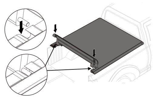
6. • Press down to close the cover and the lock will automatically clamp.
